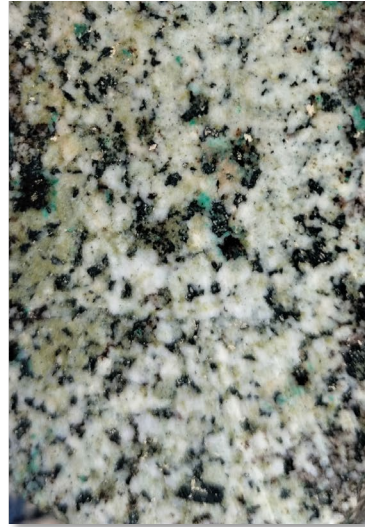
Monzonite with sericite alteration & disseminated pyrite-chalcopyrite, locally replaced by copper oxide
