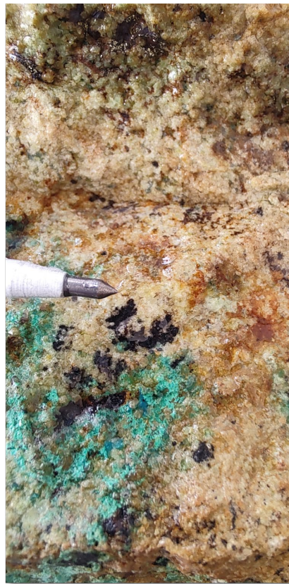
Prograde skarn alteration of garnets with supergene copper mineralization
