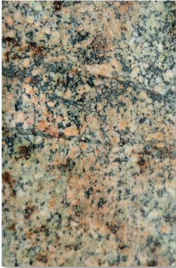
Monzonite with sericite alteration & disseminated pyrite replaced by iron oxide
