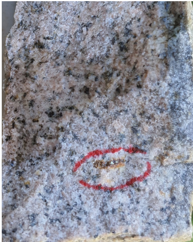
Porphyritic dacite with strong intergranular K-spar, magnetic response, sericite replacing feldspars, FeOx in veinlets and disseminations after sulphide. Chalcopyrite locally observed.
