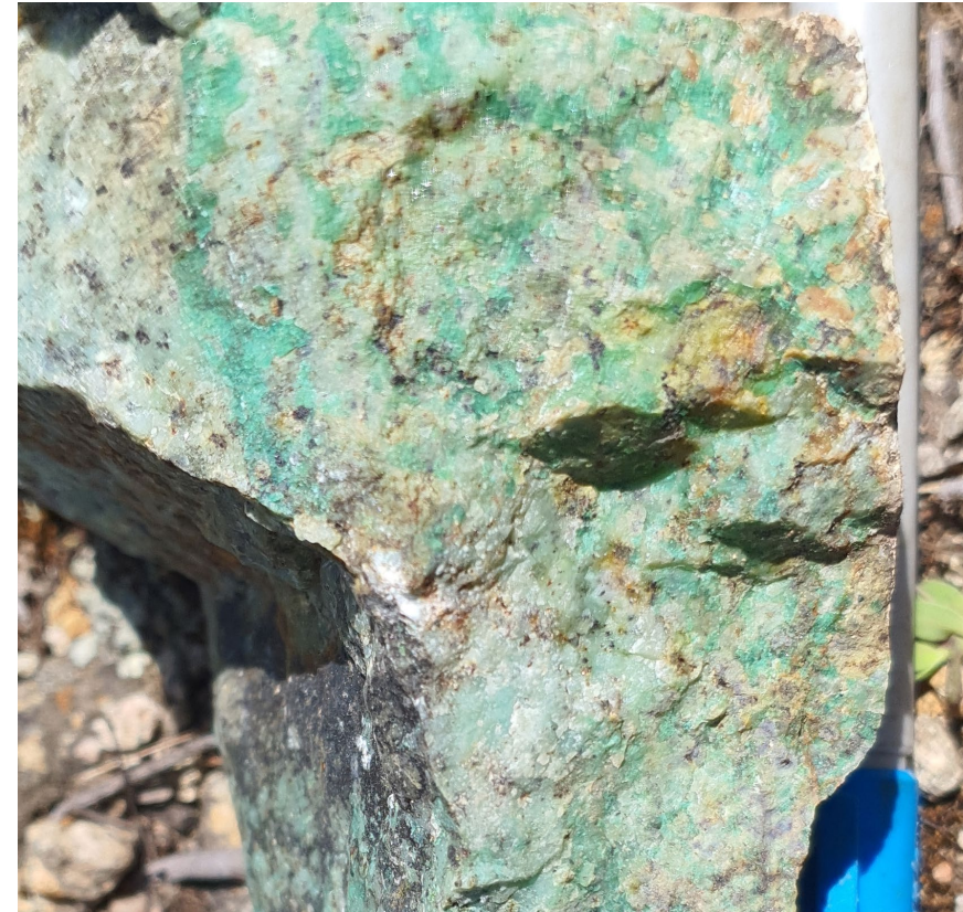
Porphyritic dacite, sericite replacing feldspars, green copper sulphates in fractures and surfaces, FeOx in veinlets and disseminations after sulphides.
