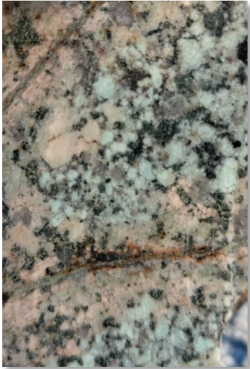
Quartz monzonite porphyry with sericite alteration cut by early dark micaceous veinlets
