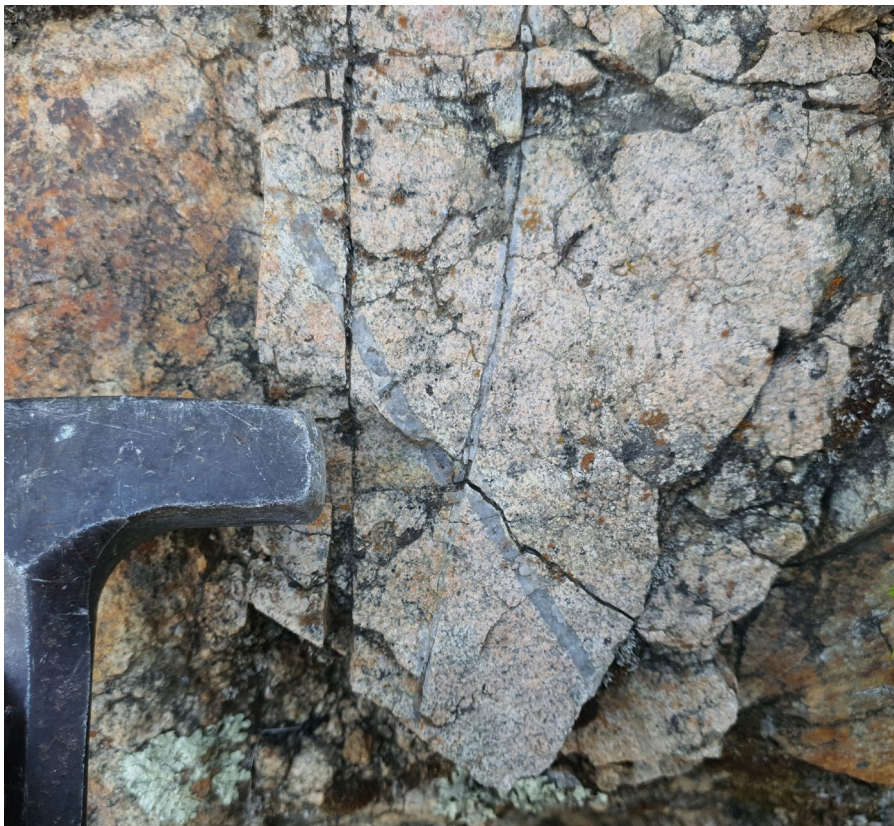
Porphyritic dacite with strong intergranular K-spar, 2 sets of quartz veinlets (B veins) up to 1cm wide, and locally sulphides in veinlets.
