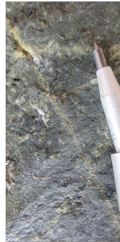
Epidote micro veinlets cutting andesite flows
