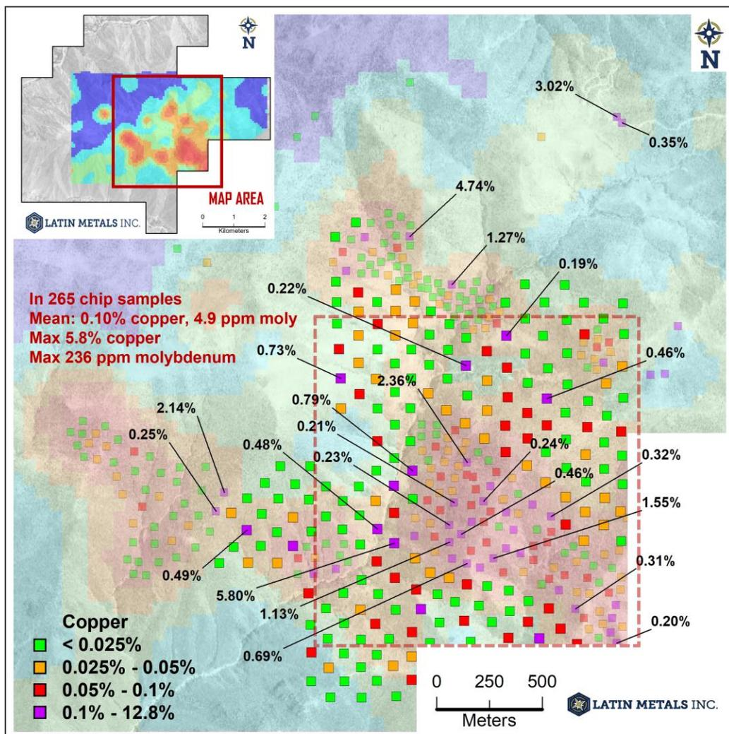
**Figure 1. Map showing all rock sample locations on the Project and highlighting rock samples not previously disclosed with a larger symbol. All copper grades greater than 0.2% copper are labelled. The area defined by red square shows consistent copper mineralization over 1.5km x 1.5km extent.**
