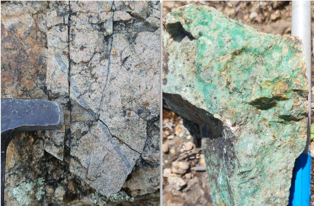
***Plate 1. Typical porphyry B-type veins in outcrop (left) and outcropping copper oxide mineralization (right) from within the core area of high-grade mineralization (shown on Figure 1).***
