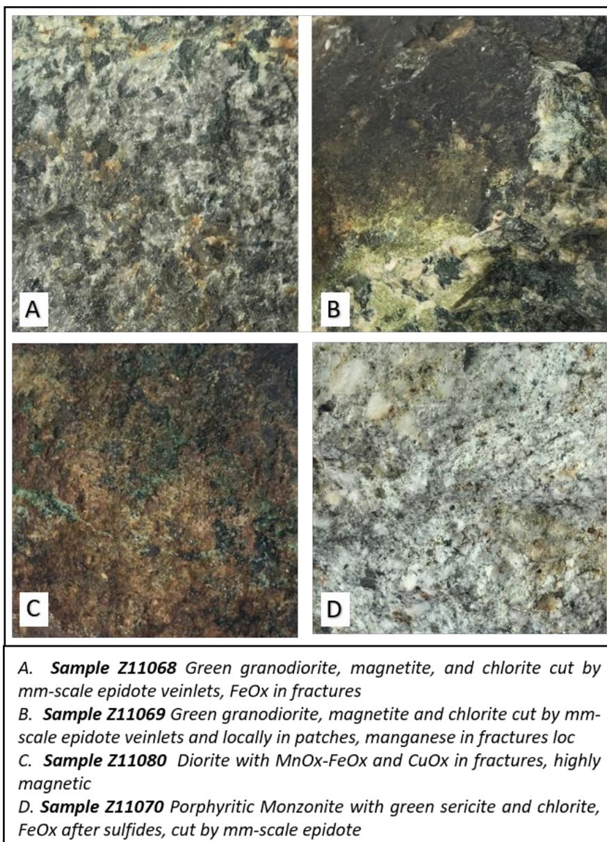
**Plate 1: Mineralized Rock Samples**
